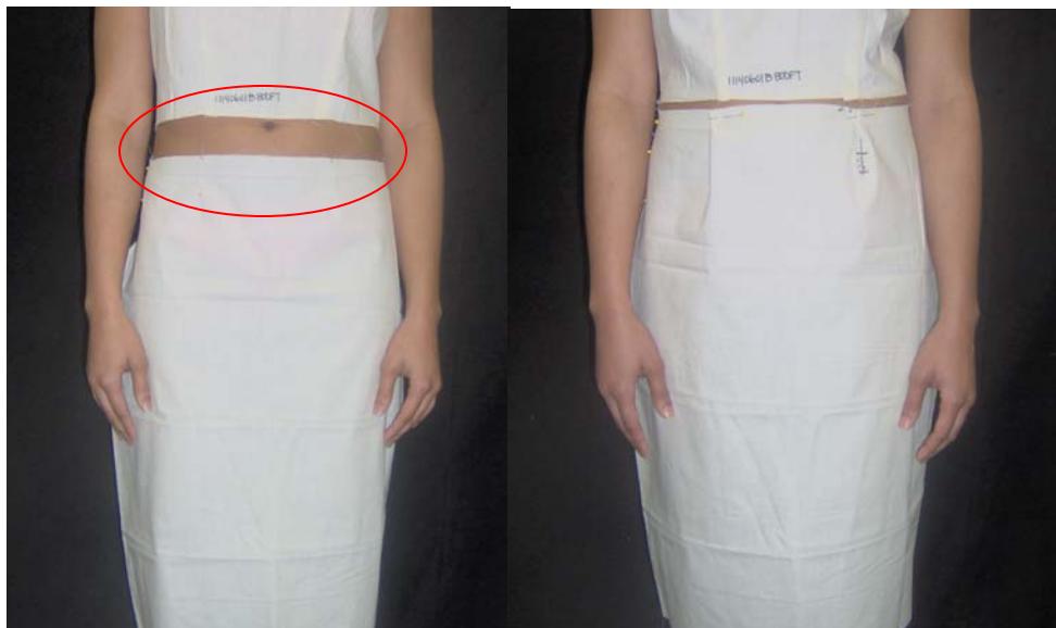
Figure 80. Skirt front dart uptake before and after.
