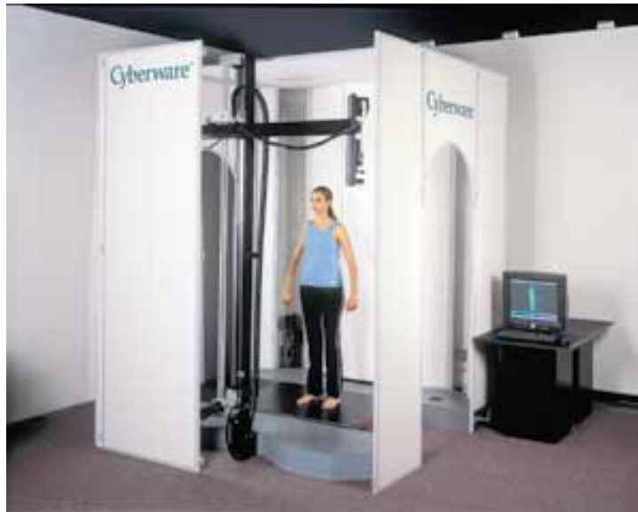
Figure 9. Cyberware's whole body X 3D body scanner retrieved from Cyberware, n.d.
