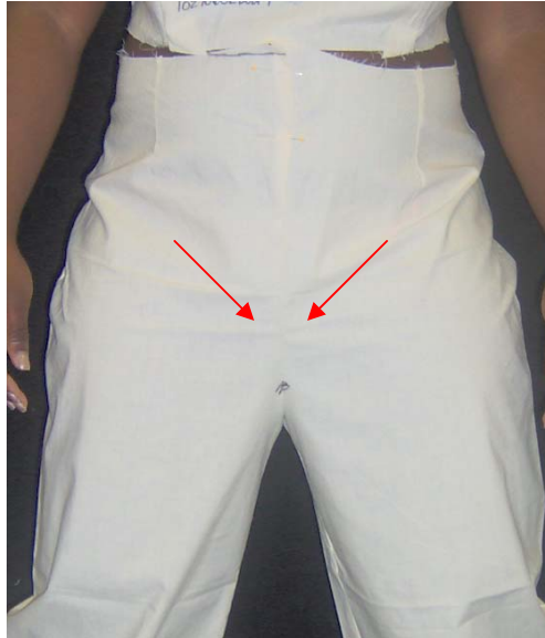
Figure 86. Pant crotch seam rise incorrect.
