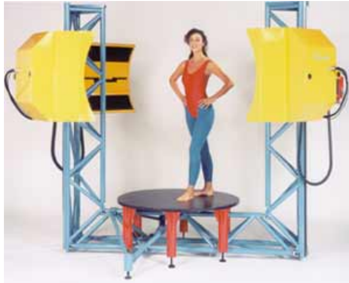
Figure 10. Cyberware’s whole body color 3D body scanner retrieved from Cyberware, n.d.
