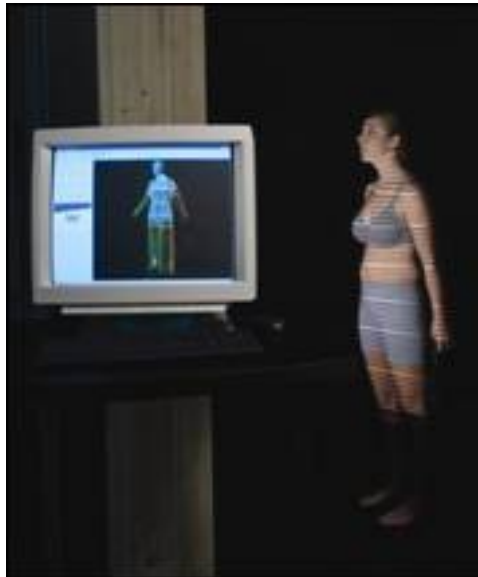
Figure 6. [TC] 2 3D body scanner retrieved from [TC] 2 , n.d.b.
