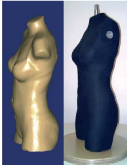
Figure 23. Mannequin developed from 3D body scan retrieved from Human Solutions, n.d.c.
