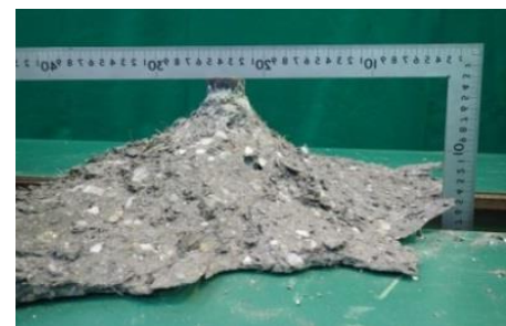
(b) Concrete cone failure
