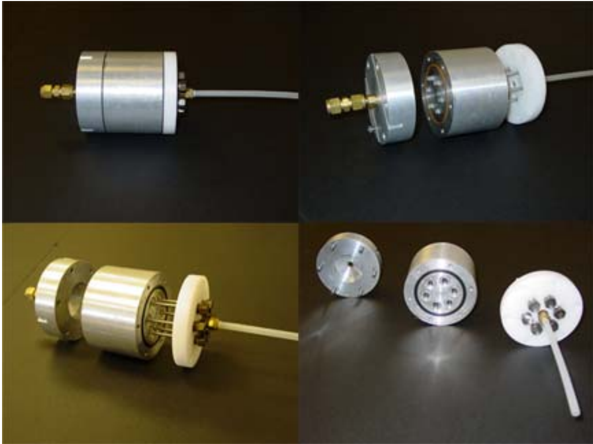
Figure 3.3: Original cylindrical DBD reactor used to process gases into renewable fuels. The reactor consisted of six independent chambers where the dielectrics in the reactor were syringes used by the medical industry.
