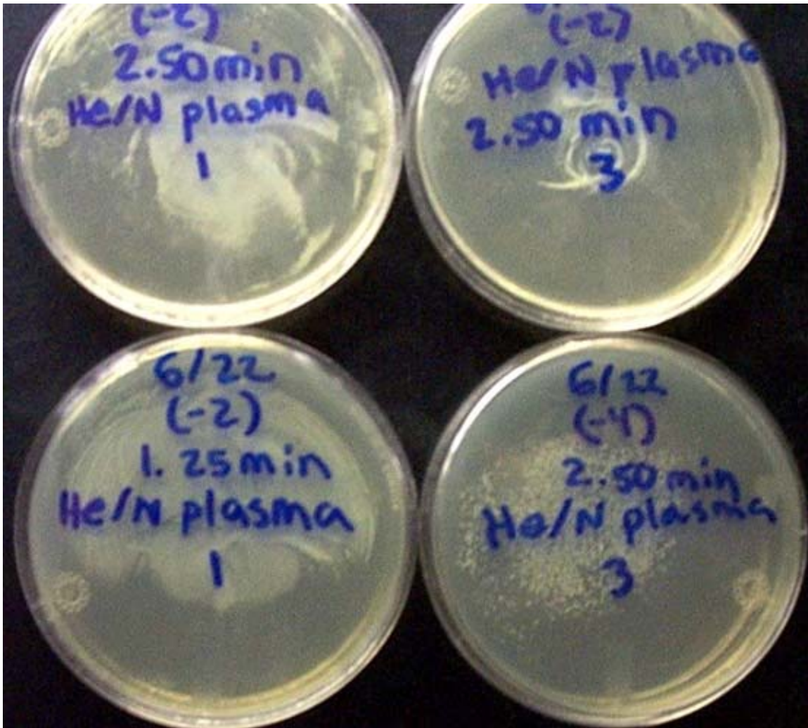
Figure 4.6: Centralized growth pattern found after 1.25 and 2.5 minute plasma exposures of 1.5% nitrogen in helium.
