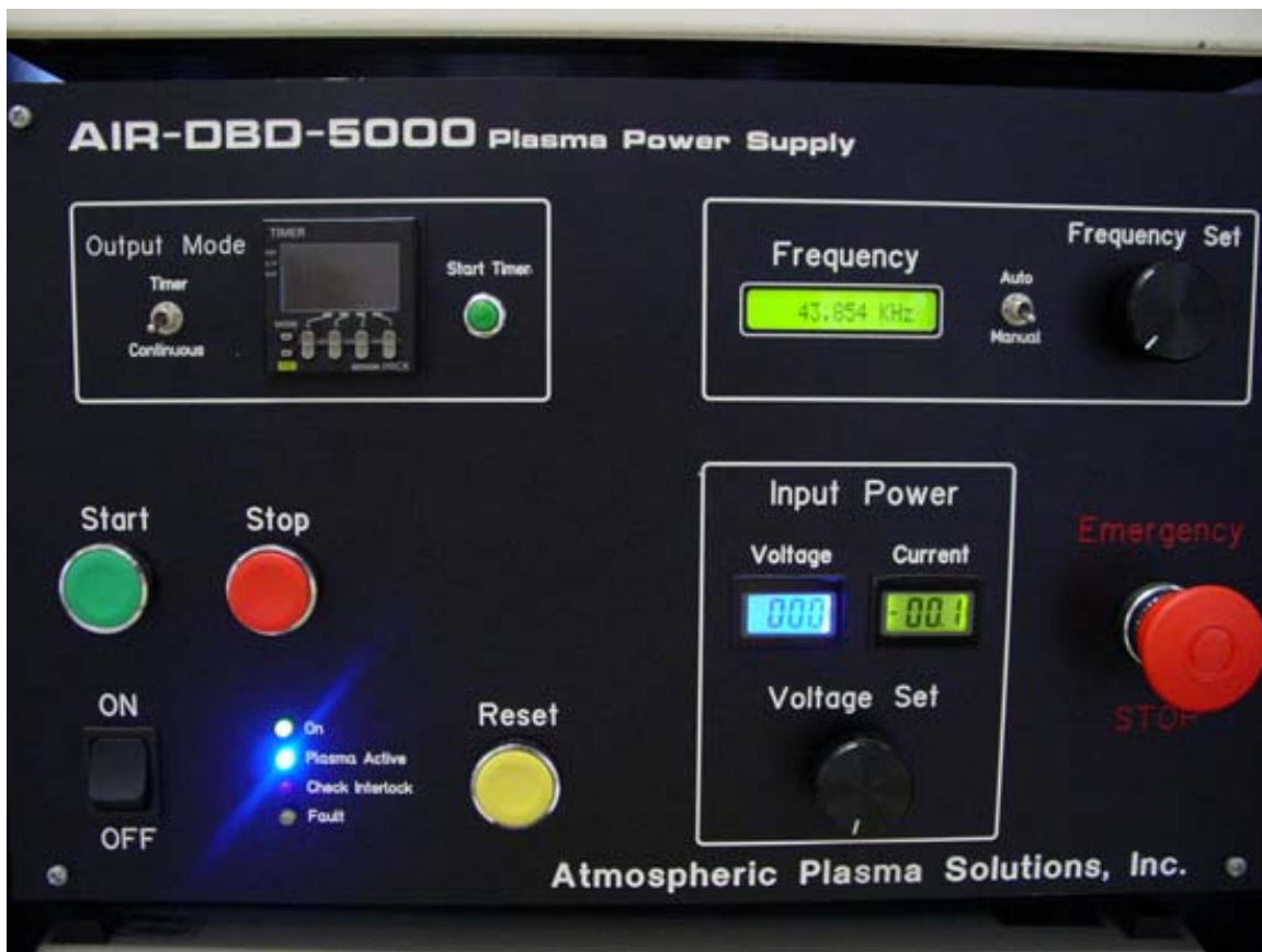
Figure 3.4: Shown in the photograph is the AP Solutions AIR-DBD-5000 power module used during the second phase of this research. Module has capability to generate up to 5000W of power.
