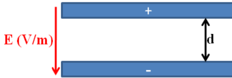
Figure 2.5: Capacitive planar discharge gap, separated by distance, d , with electric potential E .
