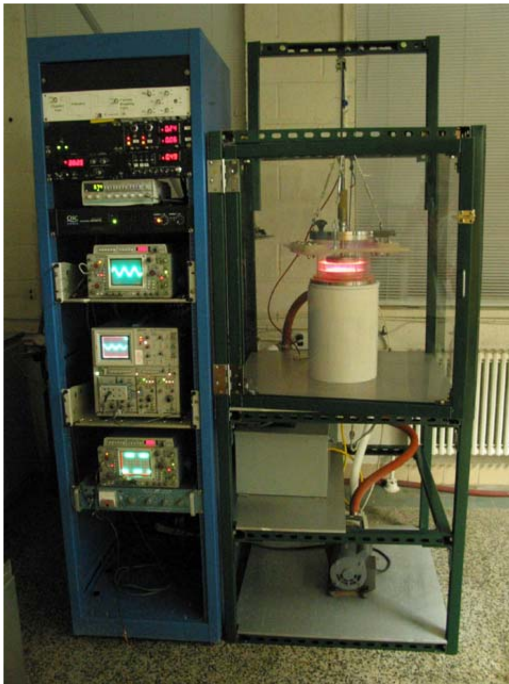
Figure 3.1: DBD reactor shown in Riddick Hall just after completing the enclosure to house the reactor, pump, and high voltage transformers. To the left is the control rack with the MOD I power supply, function generator, oscilloscopes for monitoring power, and gas monitoring and control system.
