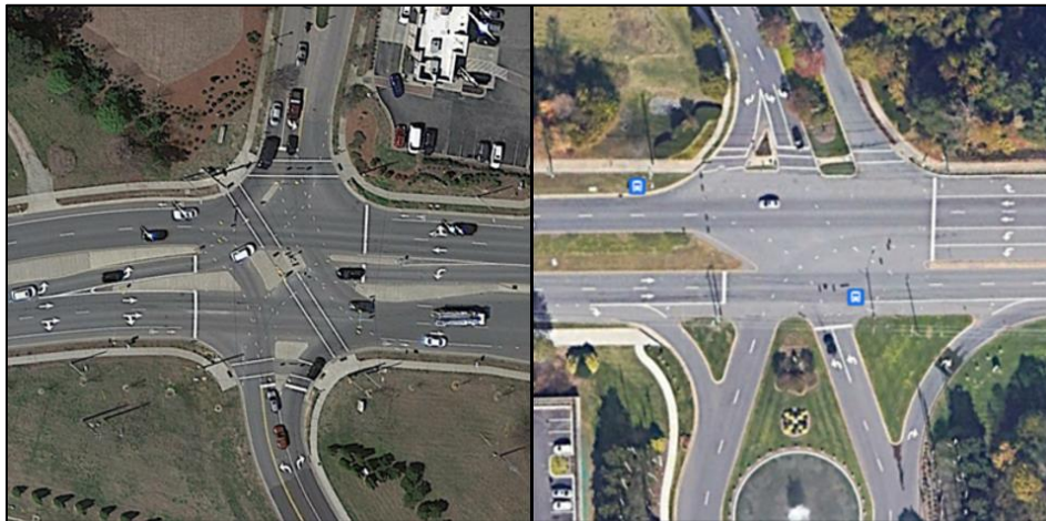
Figure 8. Thru-Cut Intersections at Village Walk Dr/S Main St, Holly Springs, NC (Left) and Arrowood Rd/Arrowpoint Blvd, Charlotte, NC (right)
