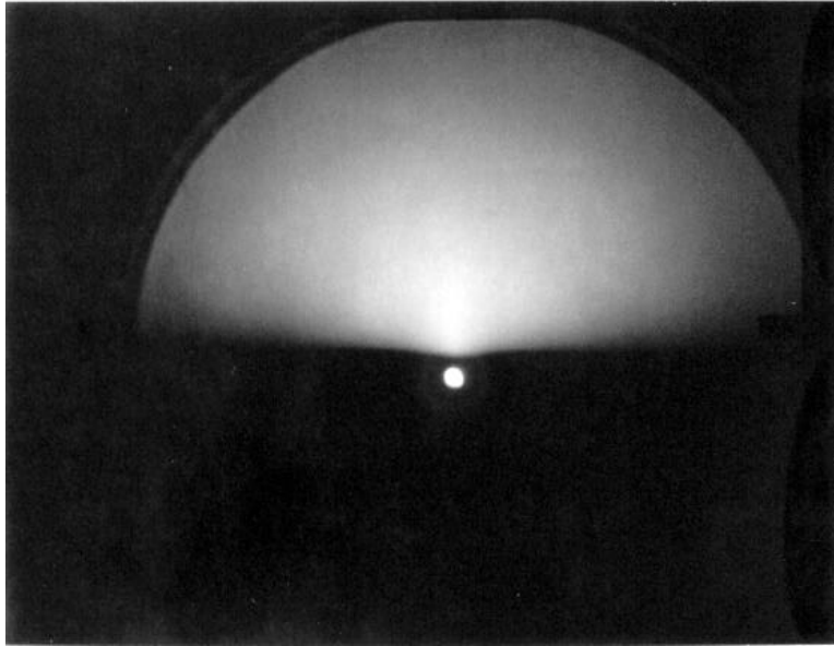
Figure 7.3.1 RHEED image of a 30 Å yttrium film on silicon remote N 2 O plasma oxidized for 60 minutes at 100 °C.
