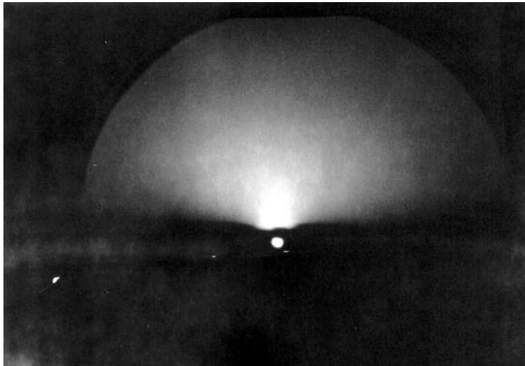
Figure 7.3.2 RHEED image of a 30 Å yttrium film on silicon remote N 2 O plasma oxidized for 60 minutes at 300 °C.
