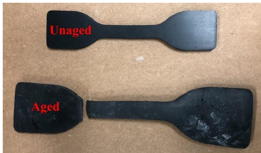
Figure 2.3 Severe swelling of CR sample after 13 weeks of exposure to benzene solution at 140 °F (Top: Unaged sample, Bottom: Swollen sample because of aging). Note: CR = chloroprene rubber.
