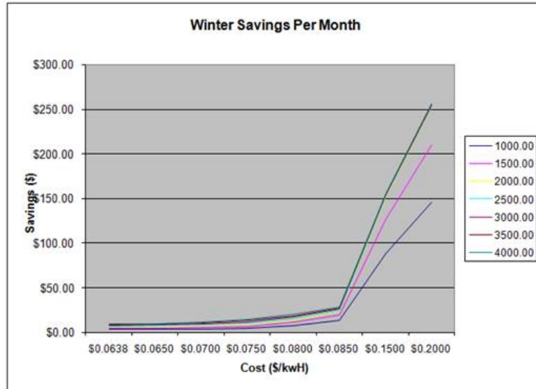
Figure 3.15: Winter Total Savings for Different Sized Households including High Rate Differences of 10 and 15 cents
