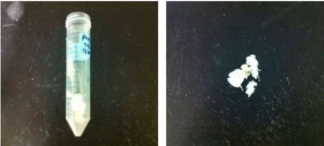
Figure 3.3 PHB pellet obtained from sugarbeet juice fermentation with partial nutrient addition media
