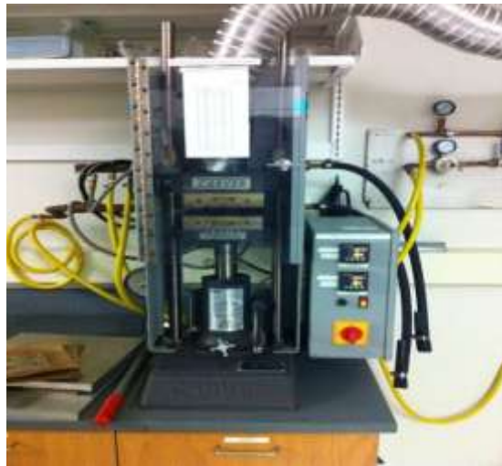
Figure 3.7 Press equipment used for samples moulding
