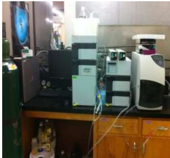
Figure 2.4 HPLC equipment used for sugar analysis
