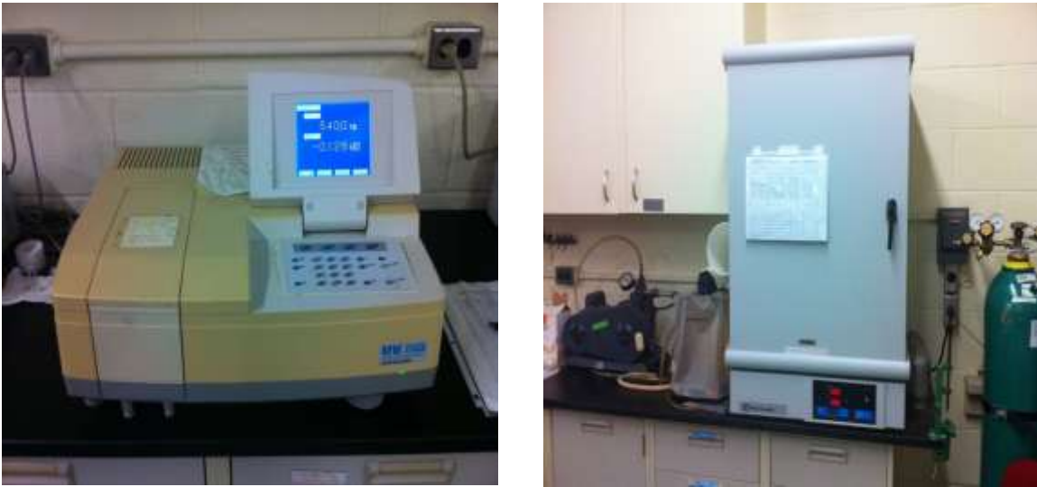
Figure 2.3 Spectrophotometer used for OD measurement and oven used for drying the cell mass
