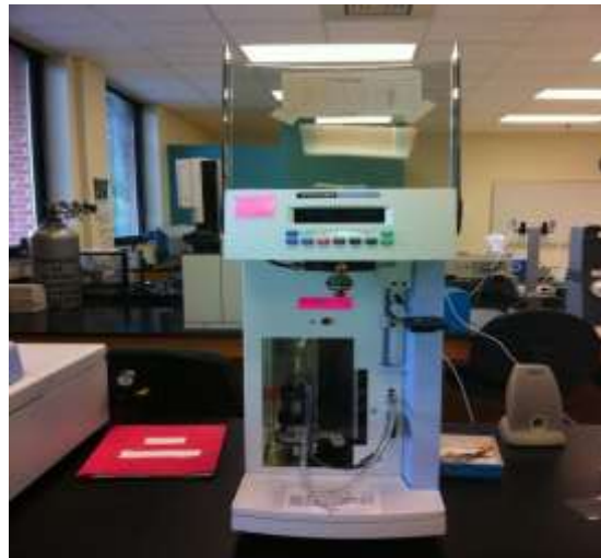
Figure 3.11 TGA equipment used in thermal analysis
