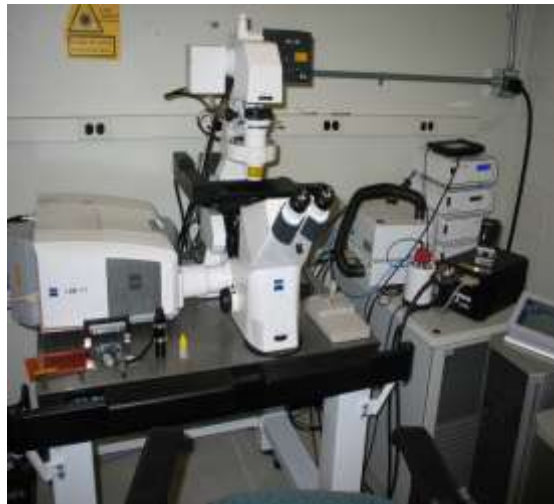
Figure 3.5 Confocal microscope used for taking images for inclusion bodies of A.latus ATCC 29714
