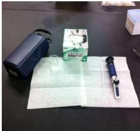
Figure 3.1 Refractometer used during sugar concentration measurement
