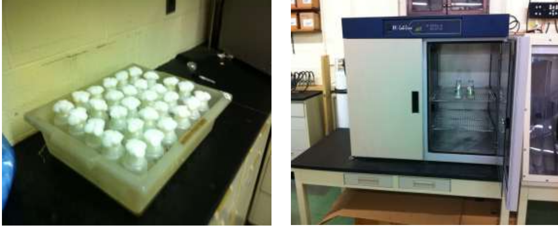
Figure 2.1 Centrifuge bottles with sponge caps used during two-stage and fed-batch culture and flasks with foil seals used for reviving culture
