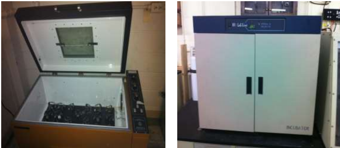
Figure 2.2 Shaking incubator used during two-stage and fed-batch culture and regular incubator used for reviving the culture
