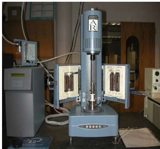
Figure 3.9 Rheometer used during rheological analysis
