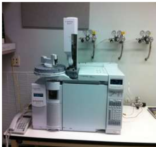
Figure 3.6 GC equipment used for PHB identification
