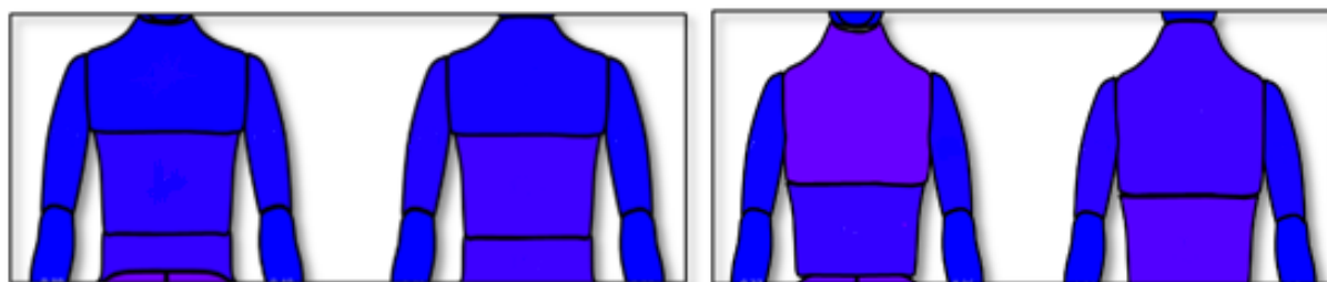
Figure 34. Thermal insulation of station uniform (SU) on male front/back (left) and female front/back (right)
