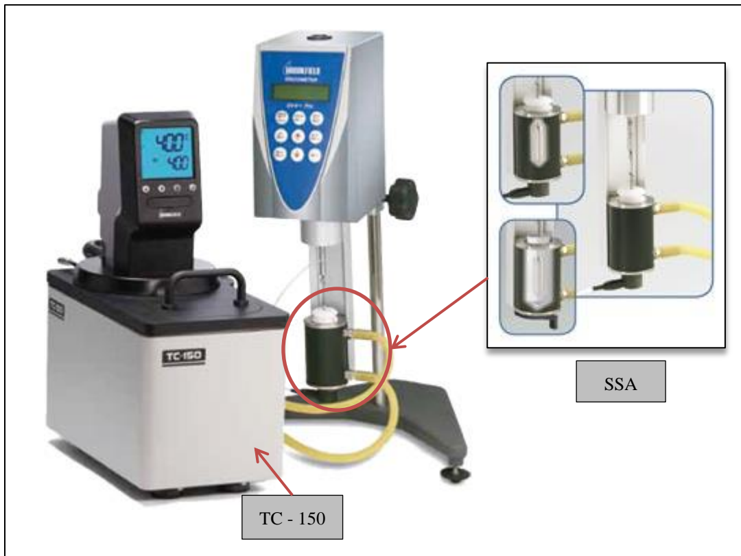
Figure 4 - 1 Rheometer setup with the SSA and temperature control bath (TC – 150)
