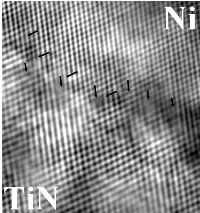
Figure 4-6 Amplified \langle 011 \rangle zone axis HRTEM image of the interface between a cube-on-cube oriented nickel island and the titanium nitride template. Small black arrows indicate extra (111) lattice planes. It is clearly seen that these are 60^\circ dislocations with a Burgers vector \frac{a}{2}\langle 110 \rangle lying in (111) planes. Some of dislocations appear in pairs combining at the interface to form a 90^\circ dislocation with Burgers vector \frac{a}{2}\langle 110 \rangle lying in (100) plane.
