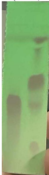
Figure 2.1: Comparison under UV illumination of GA spin-labeled(right) R_f = 5.7 cm and GA control (left) with R_f = 2.7 cm in thin-layer chromatography.
