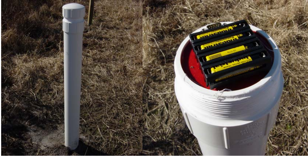
Figure 2.6 Water table well with Infinities automatic water table logger.
