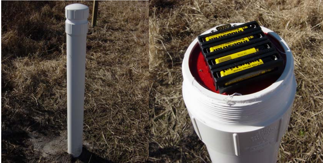
Figure 3.7 Water table monitoring well with Infinities automatic water table logger.
