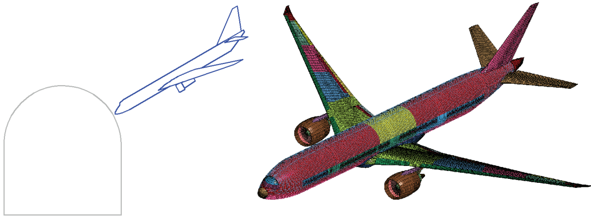
Figure 1. Impact configuration and FE model of the airplane
