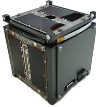
Figure 1.1: 1U CubeSat form factor [15]
