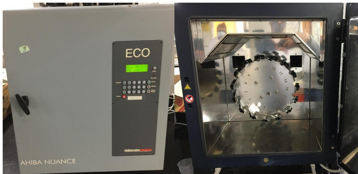
Figure 2.1. Datacolor AHIBA ECO dyeing machine (left: operation panel; right: inside of machine)
