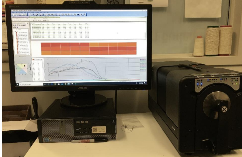
Figure 2.2. Experimental Design. X-rite Color i7 spectrophotometer and Icontrol software
