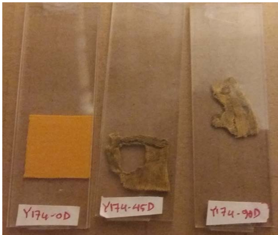
Figure 21 Photograph of degraded (45, 90 days) and not degraded R.Y 174 fabric
