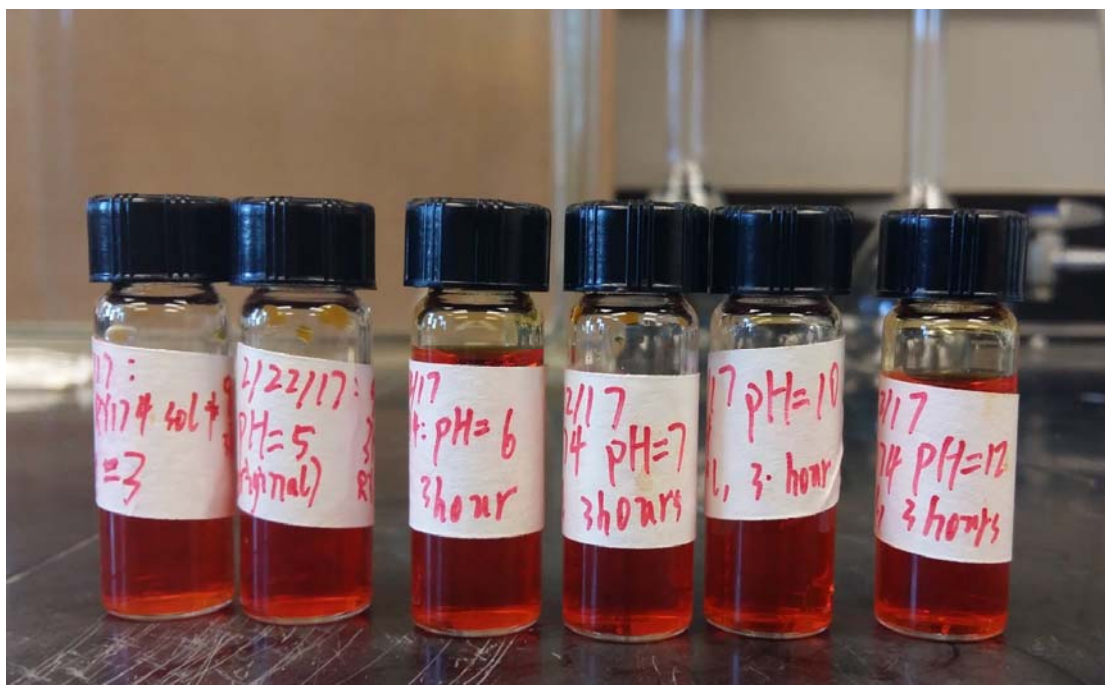
Figure 18 Reactive Yellow 174 solution heated at different pH
