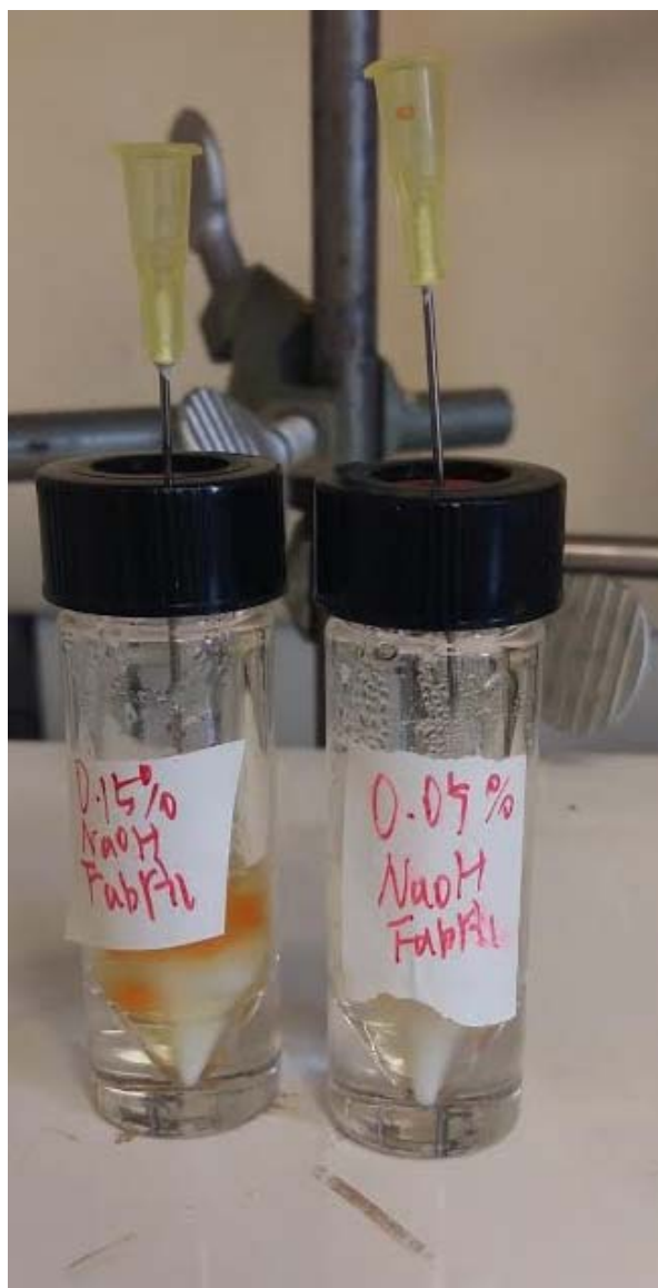
Figure 20 Setup of acid treatment experiment on undegraded Reactive Yellow 174 fabrics
