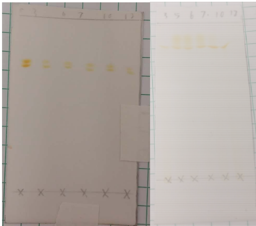
Figure 23 TLC of Reactive Yellow at different pH before (left) and after heating (right)
