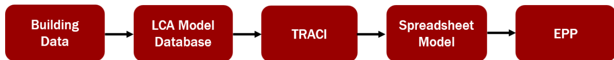
Figure 3. Environmental payback period (EPP) model workflow. Energy and material data for existing and new buildings are compiled in a life cycle assessment (LCA) model database. Impact assessment is applied using the Tool for Reduction of Chemical and Other Environmental Impacts (TRACI) method, and impact assessment results are transferred to a spreadsheet model from which EPP is calculated.
