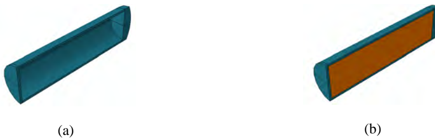
Figure 6. Sectional view of missile (a) outer shell and (b) filled with light weight concrete
