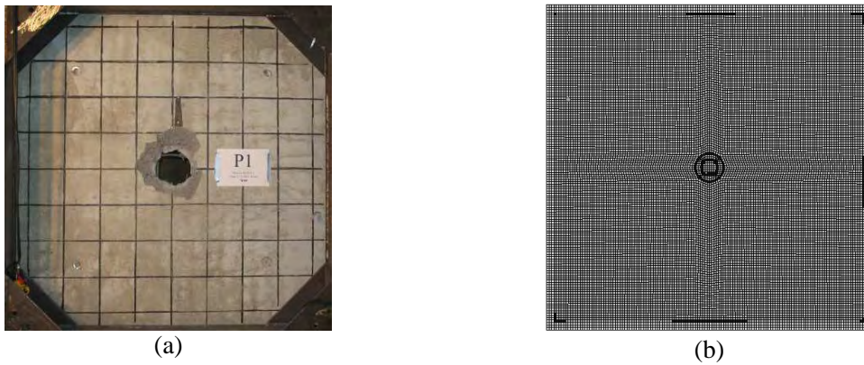
Figure 15. Spalling of target at front face; (a) experiment and (b) simulation (black areas are eroded elements)
