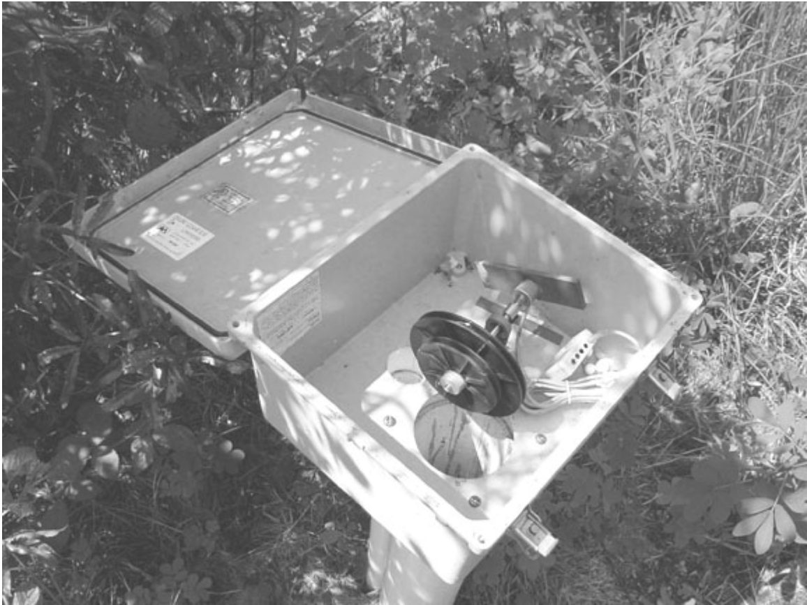
Figure 2. Image of pulley/float recording system showing the pulley, potentiometer, and the data logger
