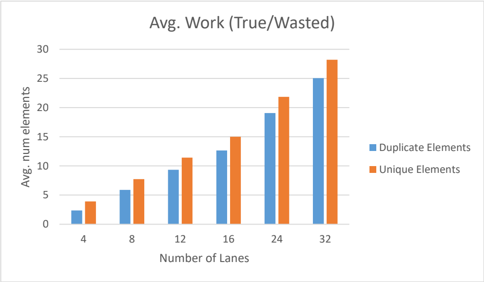
Figure 14: Average unique and duplicate elements per vector iteration
