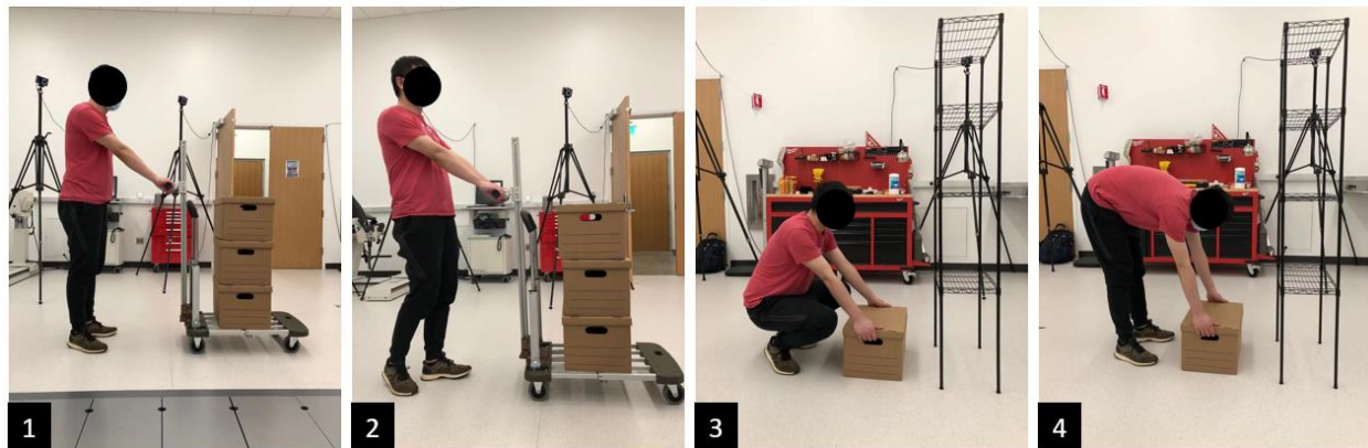
Figure 5-8 Participant performed a series of MMH movements: 1. Push the loaded handcart; 2. Pull the loaded handcart; 3. Squat lift the box; 4. Stoop lift the box. To note, the number/label of the movements were not the actual sequence of the tasks. The participants performed the tasks in the following sequence: 1 - 3 - 4 - 2.
