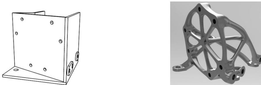
Figure 2.1 Example of topology optimization applied to a component for a space flight
