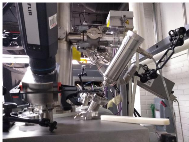
Figure 3.13 Thermal camera and pyrometer attached to the top of the Arcam S12.
