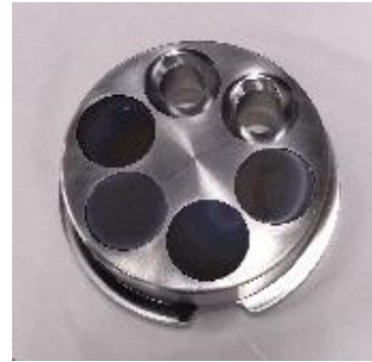
Figure 3.8 Pucks pressed at 8 MPa for 5mins, Figure 3.9 Pucks placed in the Stainless- ready to be heated. Steel baseplate at CAMAL
