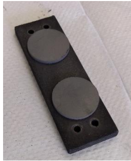
Figure 3.8 Pucks pressed at 8 MPa for 5mins, Figure 3.9 Pucks placed in the Stainless- ready to be heated. Steel baseplate at CAMAL
