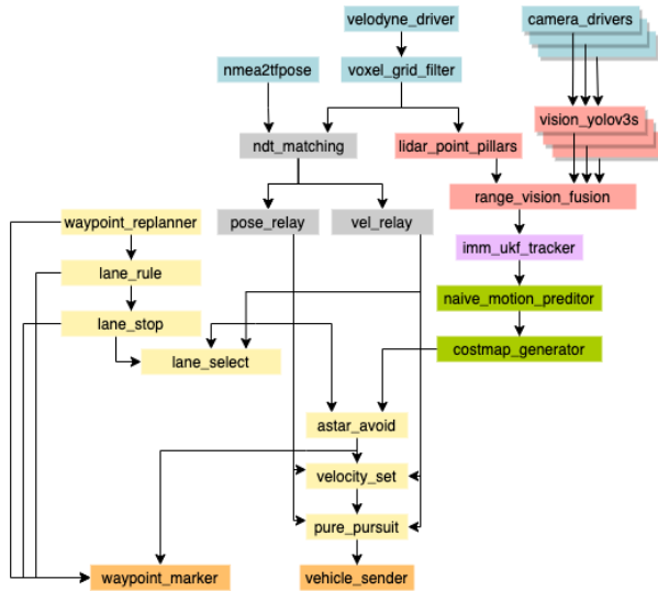
Figure 2.2: Detailed tasks within an example autonomous driving application (ADApp) derived from Autware. We categorize the tasks into the modules in Figure 2.1: Sensing (blue), Perception (red), Localization (gray), Tracking (purple), Prediction (green), Planning (yellow), and final control output (orange)
