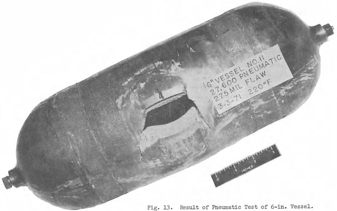
Fig. 13. Result of Pneumatic Test of 6-in. Vessel.
