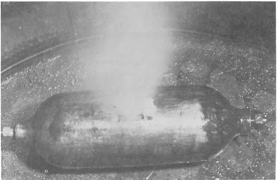
Fig. 8. 3-in. Vessel Leaking Under Pressure.
