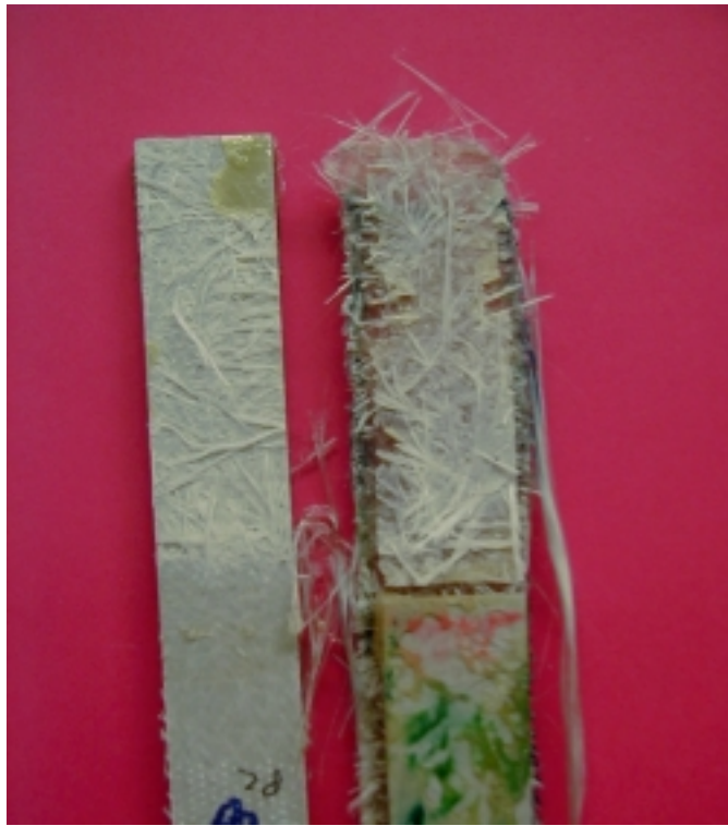
Figure 7.5: Interface after failure for specimens with ATPRIME ®
