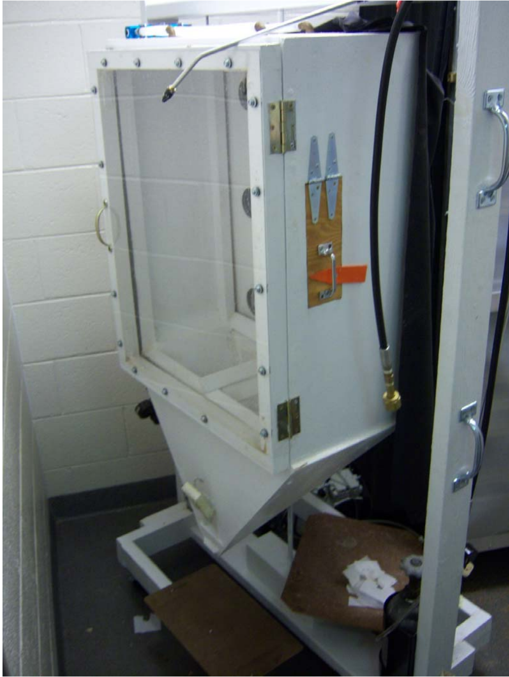
Figure 6. Carbon Dioxide chamber used to capture newly emerged moths.
