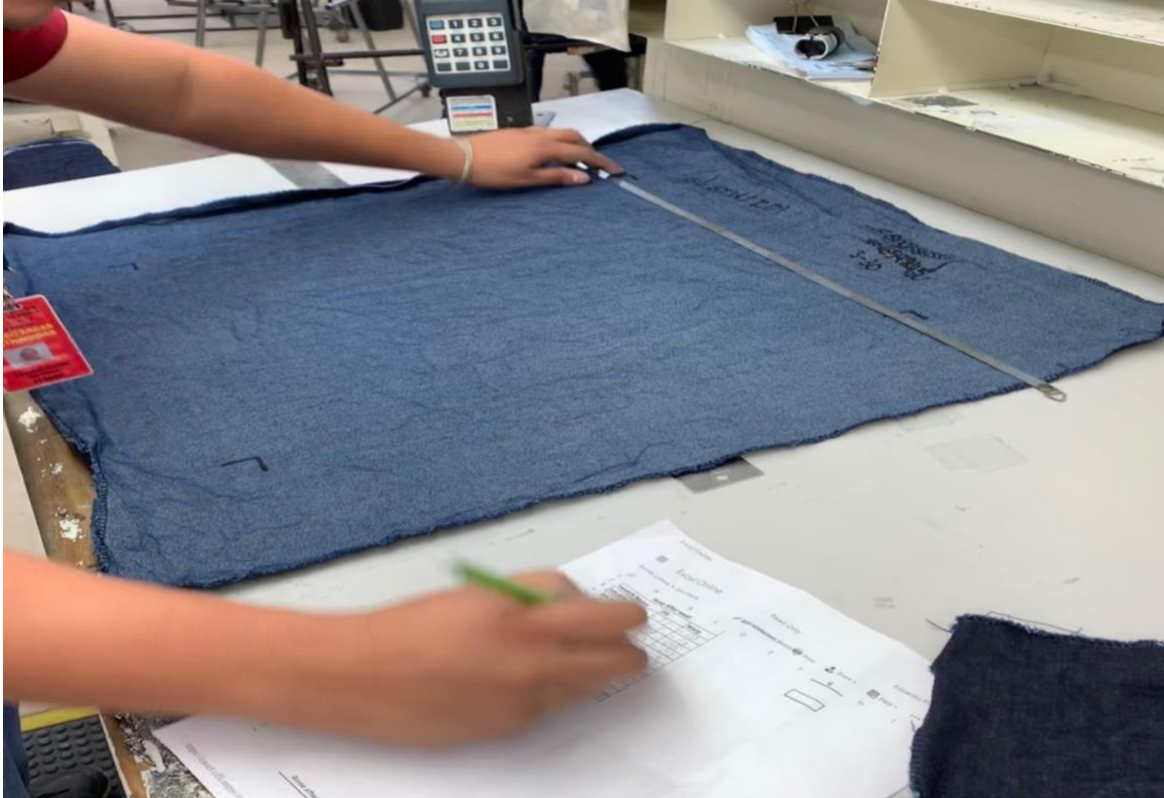
Figure 28: Image of Shrinkage Measurement of Fabric Swatches
