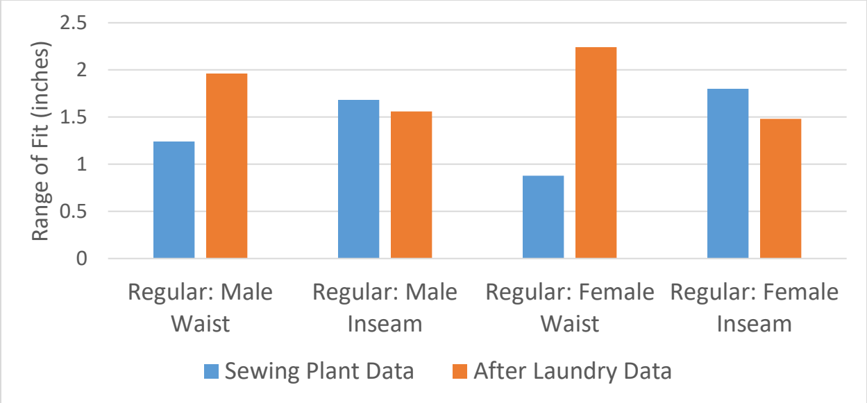
Figure 18: Range of Fit (95% CI) of Sewing and Finishing Audit Data 100% Cotton Denim
