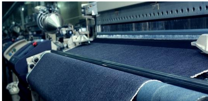
Figure 10: Weaving of Denim Fabric (“Denim and Jeans Manufacturing Process,” n.d.)
