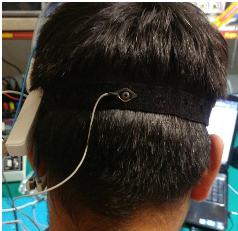
Figure 2.19 EEG wet, golden cup electrode connected to occipital lobe.
