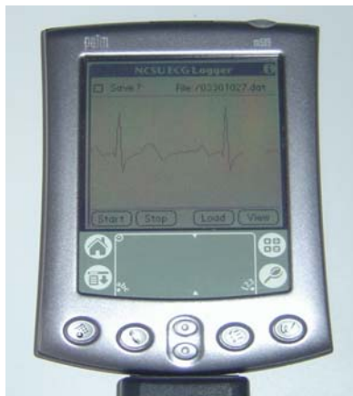
Fig. 9. Palm Pilot® displaying ECG signals in real-time.
