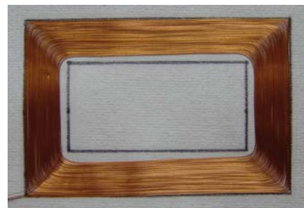
(b) Two interleaved wires wound together (four terminals, type \beta )
