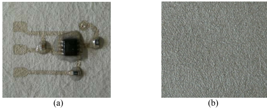
Fig. 2. Screen-printed active electrodes. a) The circuit layer with signal and power paths and components attached, b) The transducer layer filled with silver ink by screen printing.
