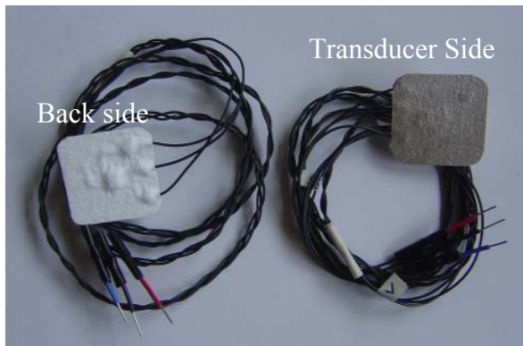
(b) Active electrodes without the guard layer
