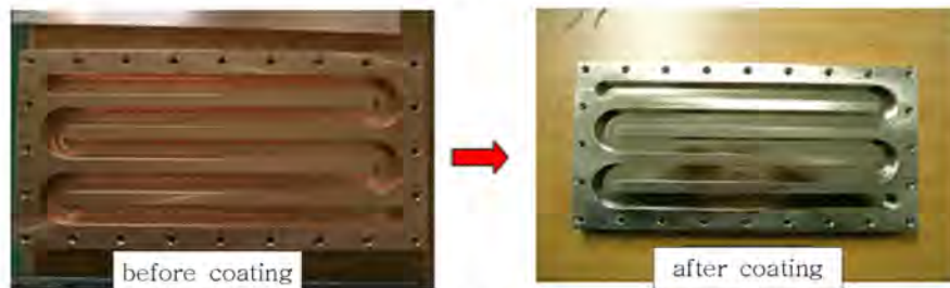
Fig.5 Copper Beam Dump Coated with Nickel
