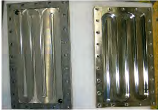
(b) Coated Surface after Erosion Test for 720 hours Fig.6 Erosion Test
