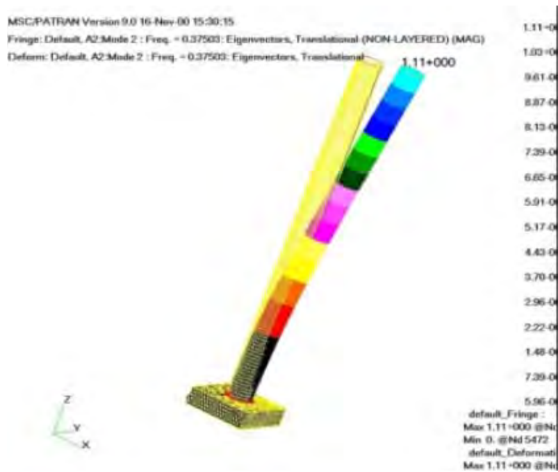
Figure 1 The lowest natural shape of the shell model. The natural frequency is 0.375 Hz
