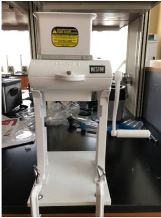
Supplemental Figure 2.1. Meat grinder used for simulated mastication of grapes (Weston Heavy Duty Meat Cube Tenderizer, Southern Pines, NC, USA). Images illustrate outcomes of whole grapes processed by human mastication (A) and that derived from simulated mastication (B) of red seeded table grapes.
