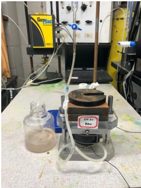
Figure 5.2 Photo and illustration of bottom-up injection setup for gravity drainage MICP treatment undergoing MICP treatment at 10 kPa confining pressure.
