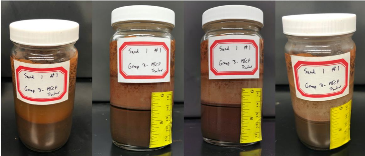
Figure 4.3 Pictures of modified self-consolidation-fall cone column tests from beginning of trial (day 0, left) to end of trial (day 7, right). Photos were also taken on days 2 and 5.
