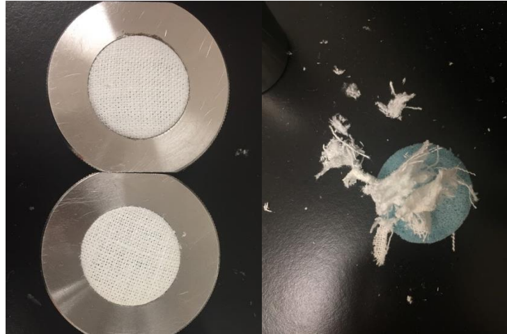
Figure 19. Hemp samples after 5000 abrasion cycles
