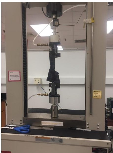
Figure 16. Cotton Woven Set-Up on Tongue Tear Tester
