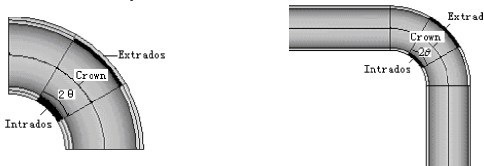
Fig.1 the sketch of cracked elbow (used in theoretical analysis) Fig.2 the sketch of cracked elbow (used in FE analysis)
