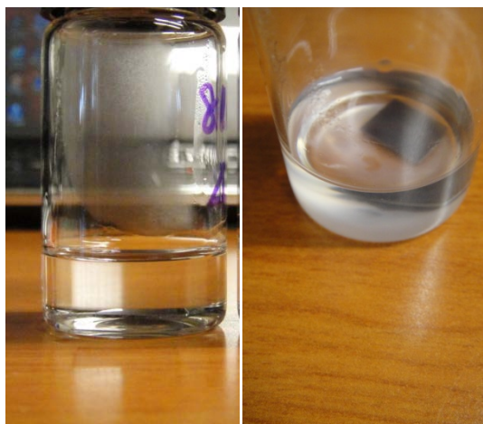
Figure 2.2.13 Photographs of the reaction vials used for the growth of PCL brushes at 25 °C for 48 h in (left )THF and (right) toluene.
