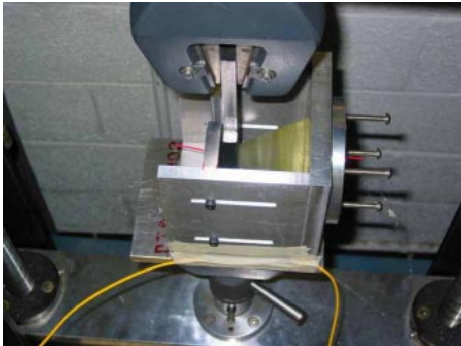
Figure 4.4: The conical epoxy specimen mounted in the loading frame. Also visible is the loading arm held in the grips of the loading machine.
