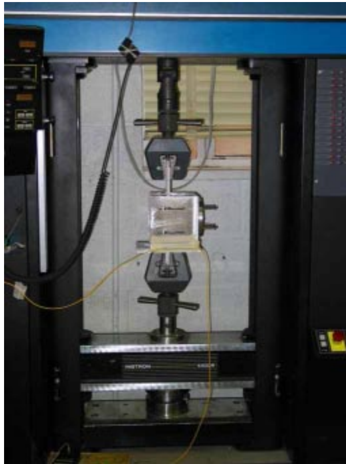
Figure 4.3: The loading frame mounted in the tensile loading machine. Also visible are optical fiber leads from the specimen.
