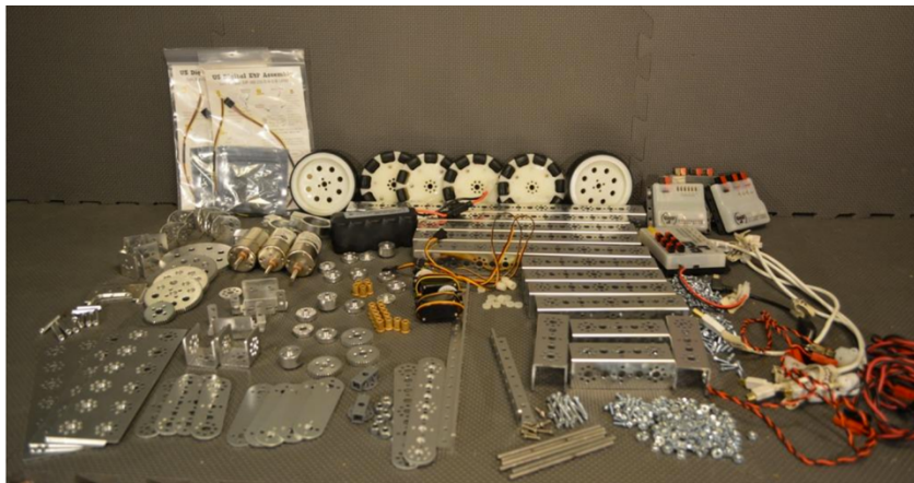
Figure 5. An example of an FTC robot kit for 2014/2015 PushBot Challenge (photo credit: unknown).
