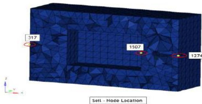
Figure 7. Soil node location around concrete chamber.
