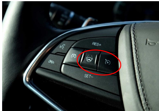
Figure 3. Super Cruise (ACC+LKA) Control Interface in 2018 Cadillac CT6. From ( https://mobilesyryp.com/2018/01/14/cadillac-super-cruise-review-learning-not-drive/ ).
