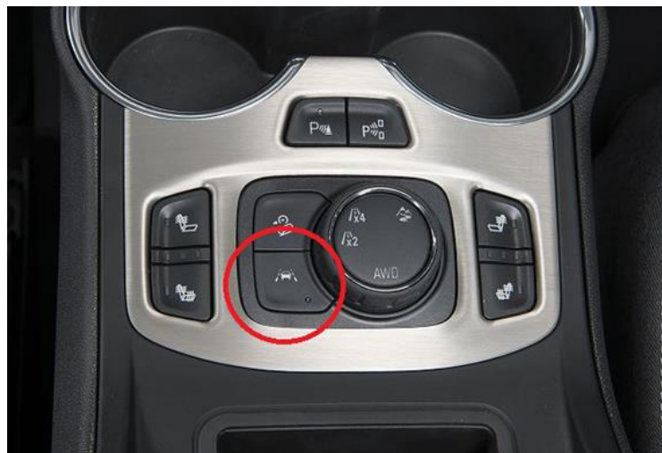
Figure 2. LKA Control Interface in 2018 GMC Terrain (From http://sandyblogs.com/techlink/?p=8224 ).
