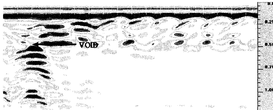
Fig. 9 Radar Measurement Result at 400 MHz(Applied Specimen)
