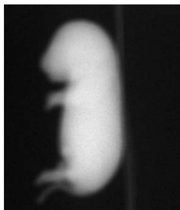
Fig. 2-26. Neutron Radiography for Mouse Fetuses
