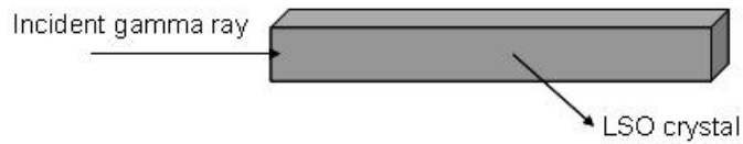
Fig. 6-6 MCNP Simulation Geometry for LSO
