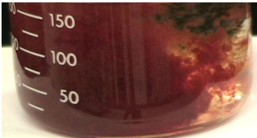
Figure 4. 59 Screen Capture of Iron (III) Hydroxide Precipitate –Susan’s “gassy fumes”
