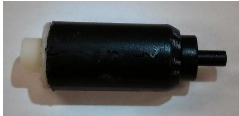
Figure 5.15: Dart Gun Charge Pressure Vessel
