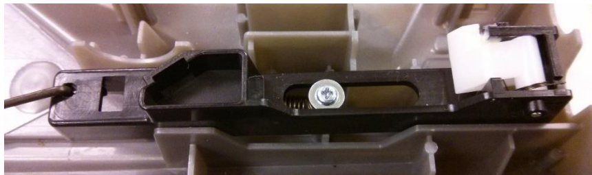
Figure 5.21: Dart Gun Trigger/Advance Assembly
