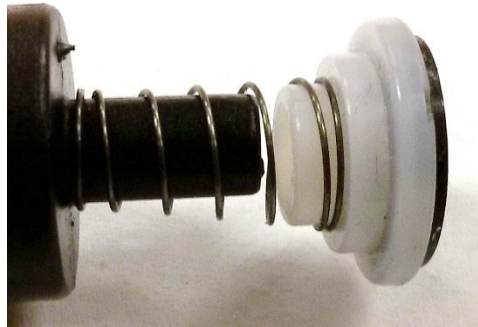
Figure 5.17: Dart Gun Floating Pressure Seal
