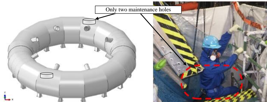
Figure 7: Accessibility to the inside of the suppression chamber
