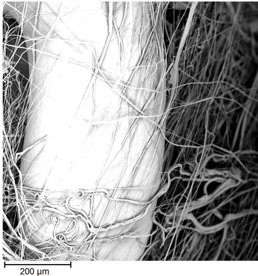
Figure 3.8 Shot particle; median diameter of fibers was 0.76 \mu\text{m} .
