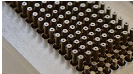
Figure 3.1 (a) Side schematic representation of the multi-row meltblowing design and fiber formation process. (b) Photo of an eight polymer row die face, with two air-only outlets at the die edge. (Photo courtesy of Biax Fiberfilm Corp)
