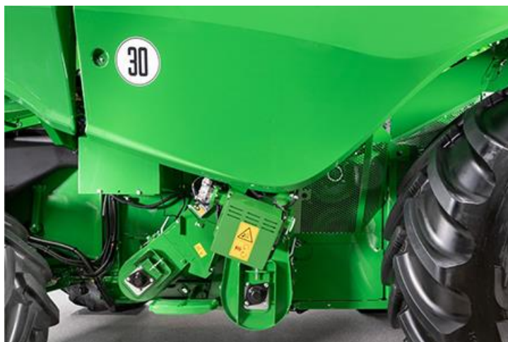
Figure 1.3 The John Deere HarvestLab 3000, an advanced agricultural technology that uses NIR spectroscopy to evaluate the quality and composition of crops at harvesting. (Deere & Company, 2023)
