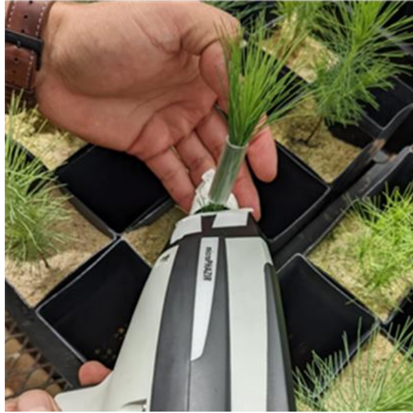
Figure 1.4 Pine seedlings, hydroponically grown, being scanned with MicroPHAZIR™ hand-held device.
