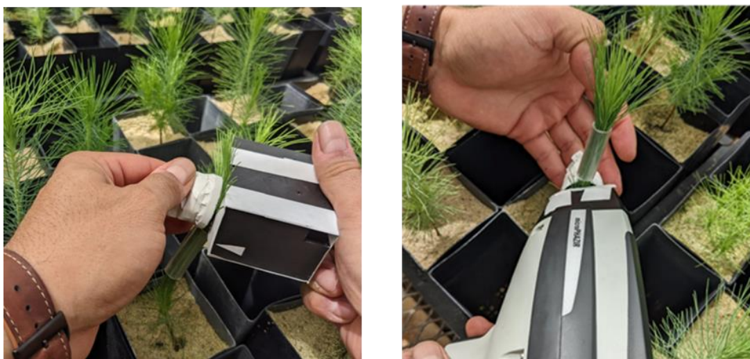
Figure 3.1 Acquisition of NIR spectra from intact pine seedlings using portable spectrometers. Left: DLP NIRscan Nano EVM (Texas Instruments) used to collect spectra from secondary needle fascicles located at the upper portion of the seedling. Right: Microphazir (Thermo Fisher Scientific) used to acquire spectra from primary needles located at the lower portion of the seedling
