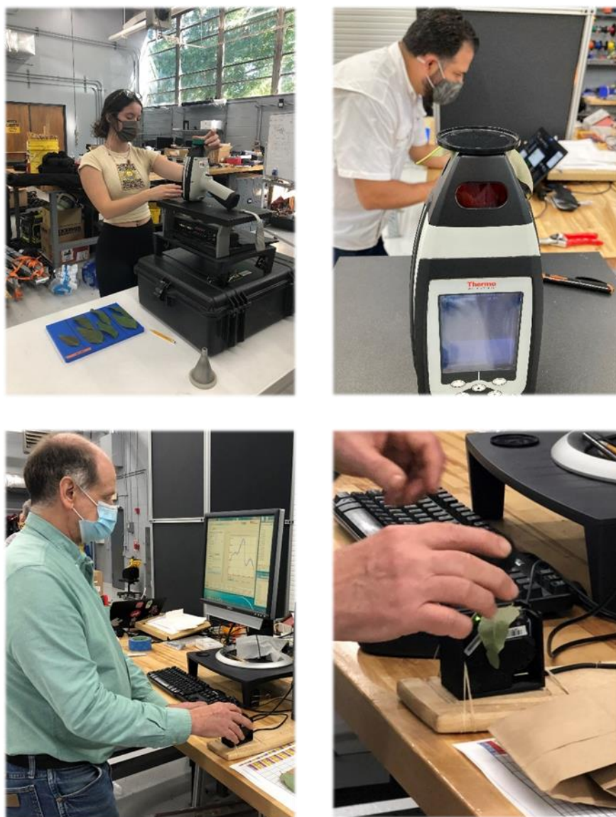
Figure 2.2 NIR spectral acquiring of eucalypt leaves using portable spectrometers. Top: Spectral measurements collected with the Microphazir scanning station. Bottom: Spectral measurements collected with the DLP NIRscan Nano EVM scanning station.
