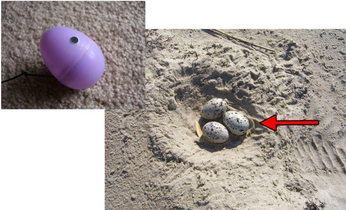
Figure 3.1. A plastic egg with an embedded microphone (left). Once covered and painted to resemble real American Oystercatcher eggs, the sensors were added to an active nest and used to record the heart rate of incubating American Oystercatchers (right). The red arrow indicates the artificial egg in the nest. The microphone is visible as a white spot on the upper surface of the egg.
