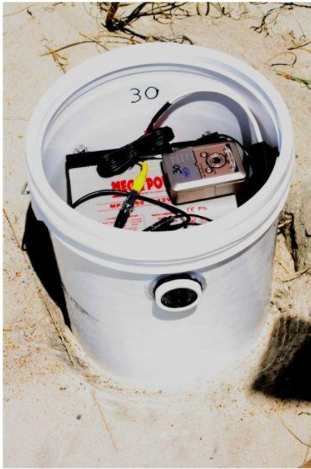
Figure 2.1. Video recording equipment used to monitor incubating American Oystercatchers and surrounding beach activity. The recording system consisted of a camera, digital video recorder, and batteries encased in a white 5-gallon plastic bucket (left). A camera unit deployed at an active oystercatcher nest at North Core Banks, Cape Lookout National Seashore, NC (right).
