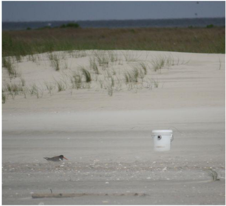
Figure 2.1. Video recording equipment used to monitor incubating American Oystercatchers and surrounding beach activity. The recording system consisted of a camera, digital video recorder, and batteries encased in a white 5-gallon plastic bucket (left). A camera unit deployed at an active oystercatcher nest at North Core Banks, Cape Lookout National Seashore, NC (right).
