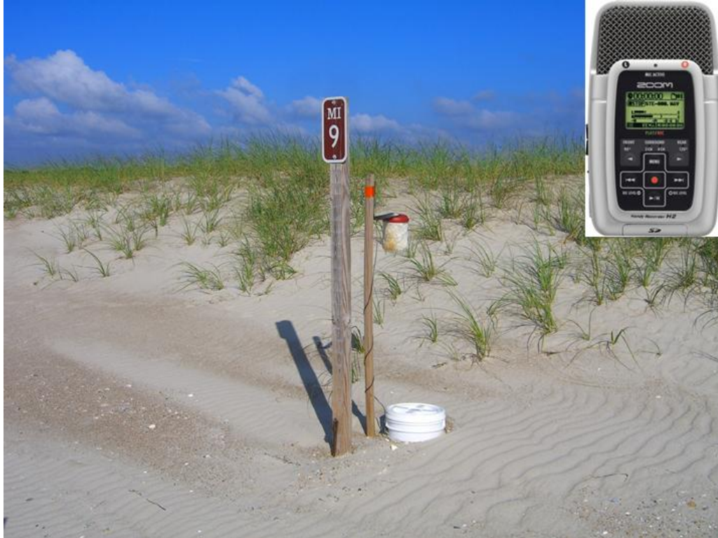
Figure 2.2. An audio recorder at mile marker nine on North Core Banks at Cape Lookout National Seashore, NC. The microphone/digital recorder (inset) is surrounded by a windscreen and suspended one meter above the ground. The white plastic bucket holds batteries that allow the recorder to run continuously for up to two weeks. An array of recorders distributed every two miles along the length of the island provided baseline ambient sound levels on the island. I also placed these recorders near American Oystercatcher nests to monitor sounds in the nesting environment.
