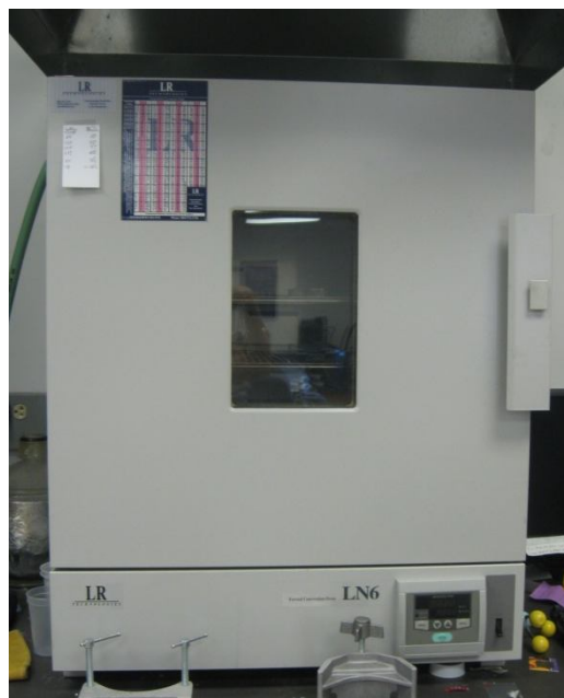
Figure 4.2 The convection oven used to thermal bond the electrospun mats
